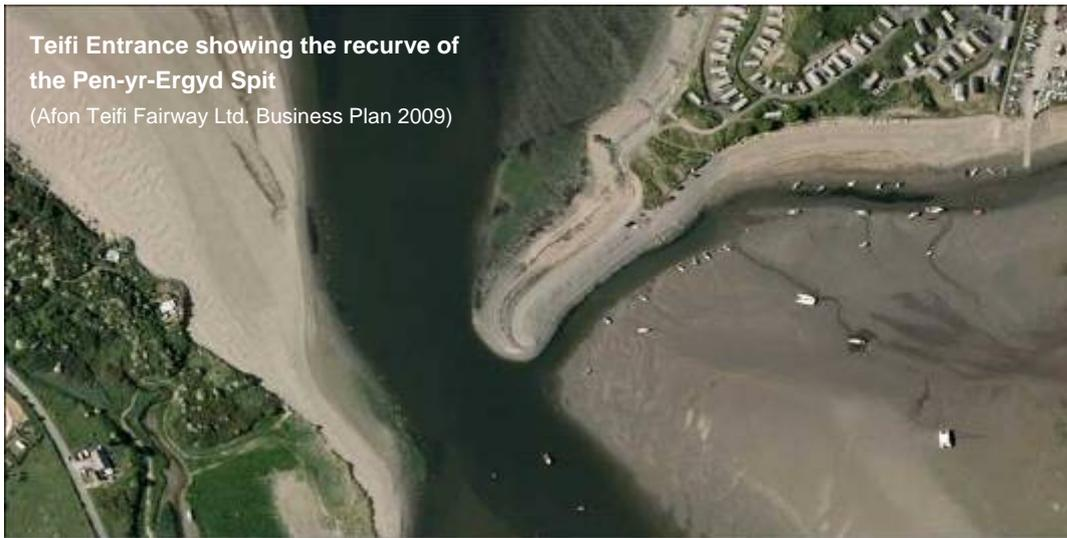
The affect of the recurve has been to further constrain flows and encourage accretion within the narrow gut-channel behind the spit, and to the fishing facility and the sailing club.
