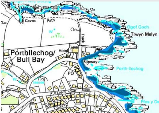
The sea front is lowest at its northern end and here there is risk of direct flooding on to the road at the critical junction providing access to properties to the north. Even under the 1m sea level rise scenario, however, direct flooding of the road would only occur on more extreme events, with flooding to a limited number of properties. Under a 2m sea level rise scenario there would be regular tidal flooding to this area of the sea front.
